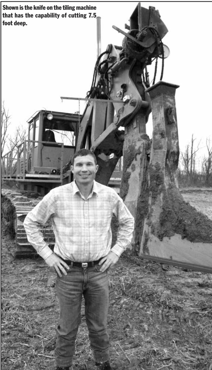
Darren explained, "we used to use perforated pipe, but the pipe would silt in after a few years and the capacity would be limited. The knife cut pipe is exactly what it sounds like, it's just as if you took a razor blade and slit the pipe." Photos by John LaRose
